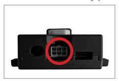
► Connect the power adapter to the MDB Interface 2.0.
